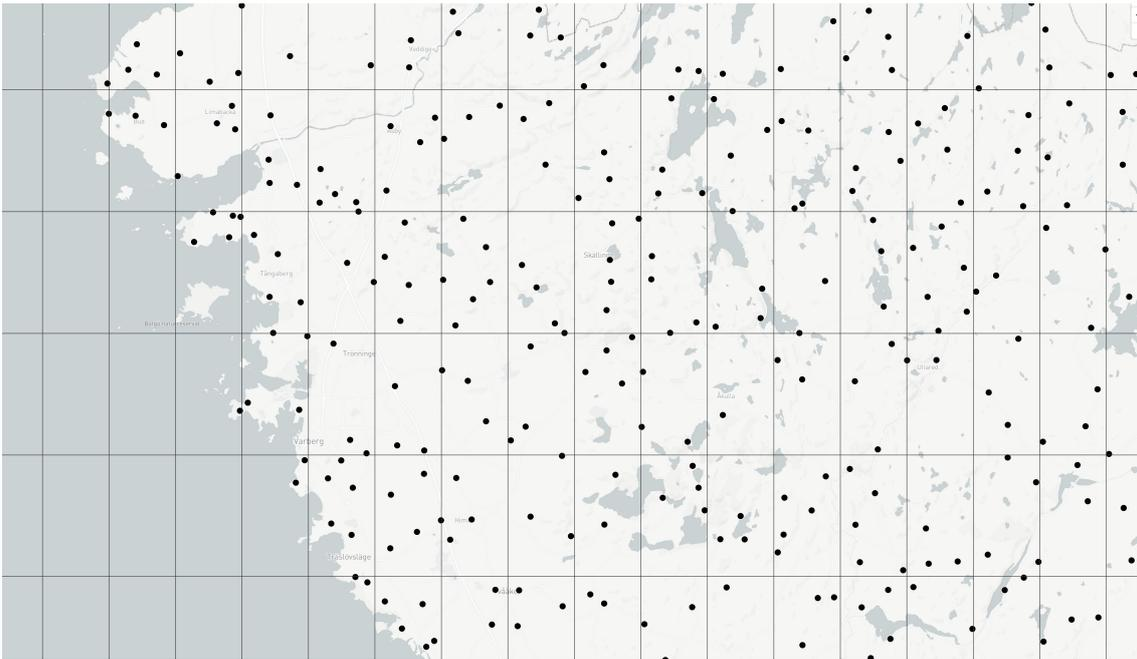
**Figure 3.5:** The grid overlay with a side length of 0.05 in latitude and 0.05 in longitude. The main purpose of using a this approach is to prevent the algorithm from choosing nodes that are too close together in a dense area, for example a city. Map © Mapbox 2020 and © OpenStreetMap 2020.
